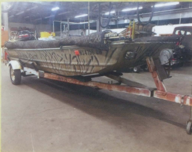
Nice and short! Vica reduced the size of the boat trailer by 16 inches to fit the boat perfectly. Kevin Kitchen said "It was fun and we got the metals class involved."
